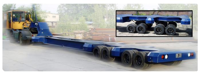
The Novatech Flexmaster is one of the most flexible and modern machines for handling standard and maxi cassettes.
